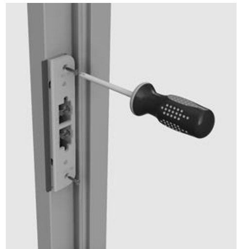
Figure 3 – Mounting the strike plate
