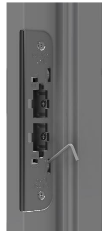
Figure 15 – Adjusting the strike plate
